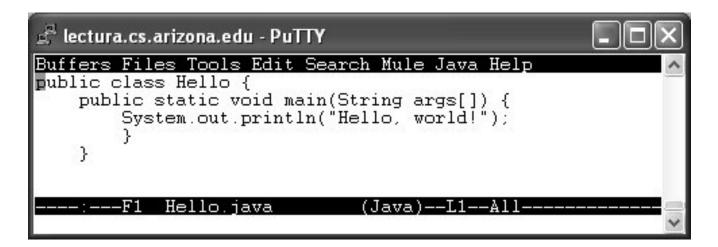
The contents of the file are loaded into a *buffer*, which is displayed in an Emacs *window*.
