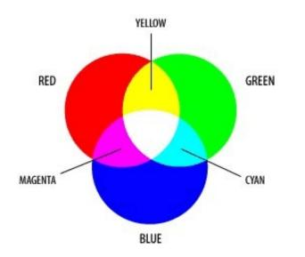
The CMY color model is commonly used when printing colors. It is called a subtractive model because ink is used to subtract colors from the image. The colors cyan, magenta, and yellow reflect no red, green, or blue light, respectively.
