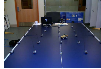
Fig. 5. Acoustic tracking experiment with a 5 \times 5 grid layout.
