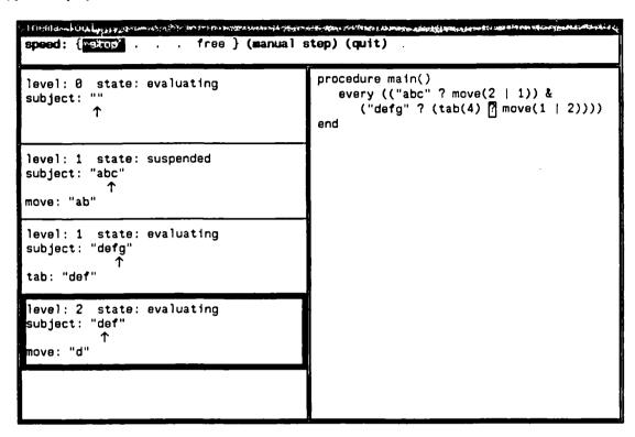
The top portion of the display is an options menu that allows the user to control Cinema. The right portion contains the program, while scanning environments appear at the left.
