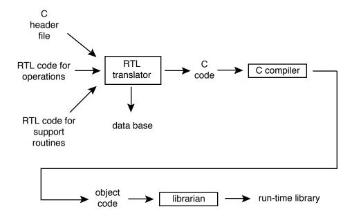
The Icon compiler produces an executable program from Icon source code by translating Icon procedures into C functions, supplying a C main function, and compiling and linking these functions with the library produced using rtt. The compiler makes use of the data base when performing the translation:
