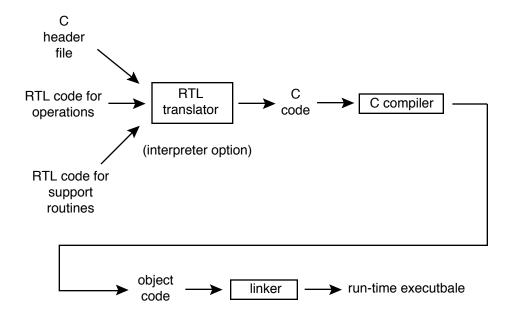
For the interpreter, Icon programs are translated into an intermediate form, which is then interpreted by iconx. iconx's interpreter loop calls the operations and support routines in the run-time system as needed.
