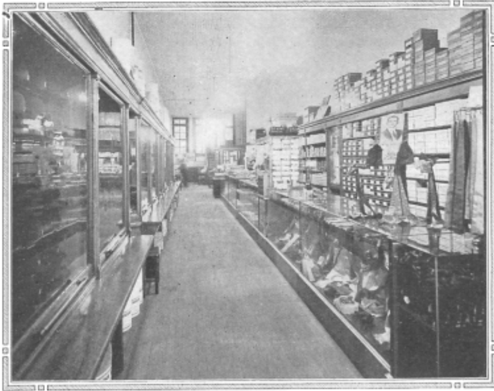
STORE WELL LIGHTED BY INCANDESCENT GAS MANTLES PROPERLY PLACED.
