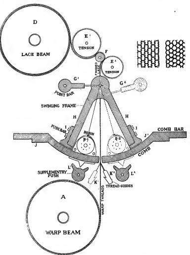
FIG. 6. SECTION OF LACE MACHINE CONE-THIRD FULL SIZE.
