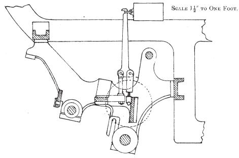
For pressure on pressing roller. Proportion of levers— Arm of pressing roller =  $l\frac{1}{2}^{"}$ . Arm of weight = 10".
