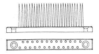
$\begin{array}{l} 10'' \times 5'' \mbox{ Roving Gill.} \\ 2\frac{7}{8} \times \frac{3''}{8} \times \frac{7}{32} \mbox{ Brass.} \\ \mbox{ 6 pins per inch.} \\ 2\frac{1''}{8} - 2 - 13. \mbox{ No. 16, 1''.} \\ \mbox{ Gill Rivet, 1'', No. 11.} \end{array}$
