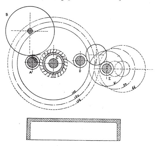
Note — The surface speed of the Rotary Gill at the point of the pin is almost equal to the surface speed of the Retaining Roller.
