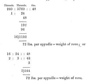
If the rove weighs 70 lbs. per spyndle, and you wish to spin 10 lbs. yarn this means a draft of 7 will be required on the Spinning Frame.
