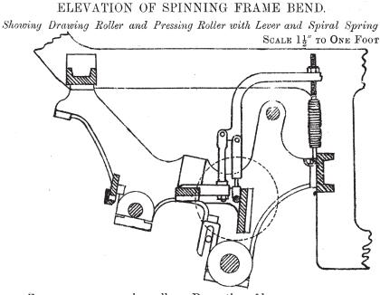
For pressure on pressing roller. Proportion of levers---Arm of pressing roller =  $1\frac{1}{2}^{n}$ . Arm of spring =  $8\frac{1}{2}^{n}$ .  $1\frac{1}{2}$ 1 Ratio  $\frac{2}{8\frac{1}{4}} = \frac{2}{5\cdot 6}$  and if pull of spring = 12 lbs. then—
