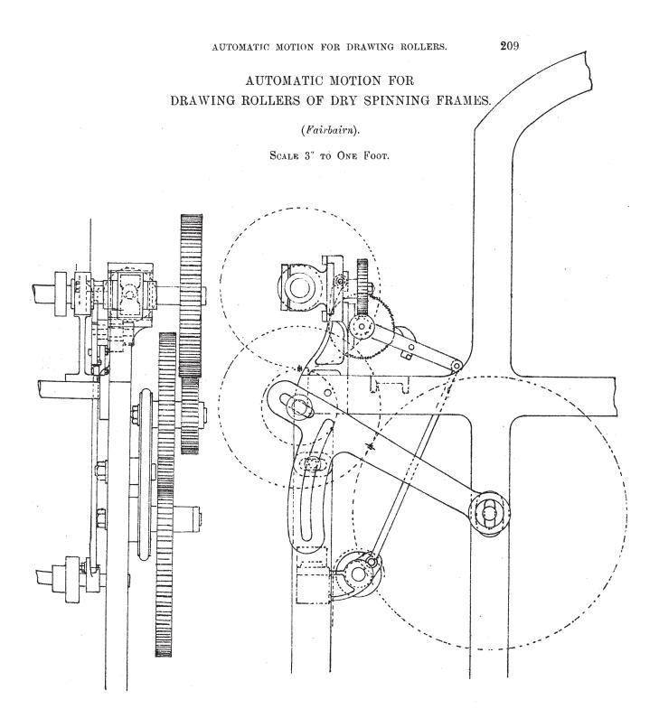
Note.—The movement of drawing roller end ways is  $\frac{1}{4}$ " in each direction.
