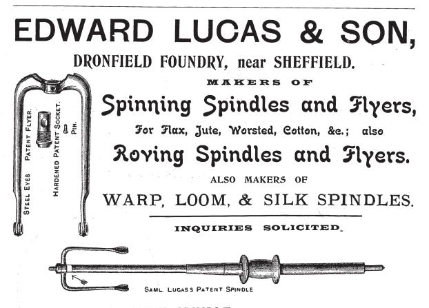
SAML. LUCAS'S PATENT SPINDLE has a collar hardened and fixed under the screw, which can be replaced; and Spindles worked down at the shoulder can have this Patent Collar put on at a small cost. The advantage of this Collar is that it prevents the shoulder at the bottom of screw becoming untrue by the flyer coming down on shoulder when working, the collar being equal in temper to the flyer. Many thousands of these Patent Spindles are now running, and are much approved.
