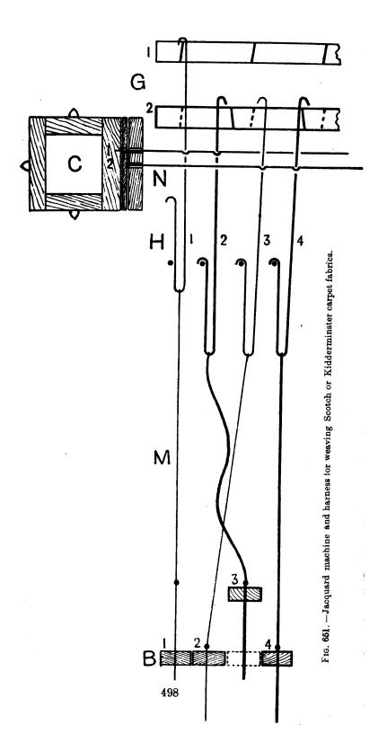
design; and also by means of comber-boards B, by which the warp threads are raised in a prescribed order according to the method of interweaving the warp and west for the creation of texture, as distinct from the scheme of decoration.
