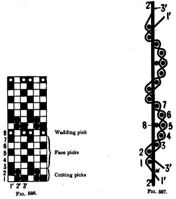
The four examples of piqué fabrics just described contain only one cutting pick each to form the furrows between the ribs, but the majority of piqué fabrics have two cutting picks inserted, in order to produce deeper and better defined furrows. Fig. 586 is a design for a piqué fabric containing eight picks to each rib, with two cutting picks, five face picks and one
