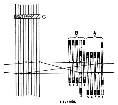
Fig. 558.—Compound presser harness for damask weaving.
