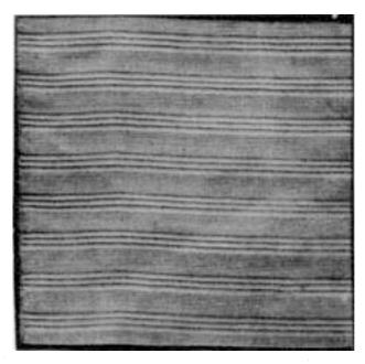
Fig. 597. -Piqué fabric with variegated welts or ribs.
