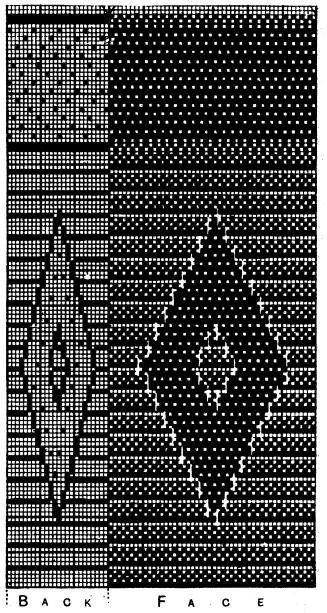
Fig. 607. -Applied design for figured piqué fabric, Fig. 606.
