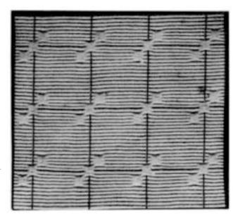
Fig. 603..-Piqué fabric figured by "floating" face warp threads; also by coloured warp and weft threads.
