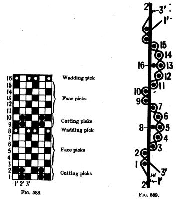
out, the complete repeat of the working design would comprise two ribs and, therefore, sixteen picks, as indicated in the design, Fig. 588, and also in the sectional diagram of the cloth, Fig. 589.
