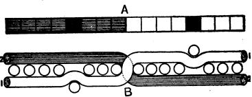
Fig. 645. —Transverse section of tapestry fabric containing one series of warp threads and two series of picks of weft.
