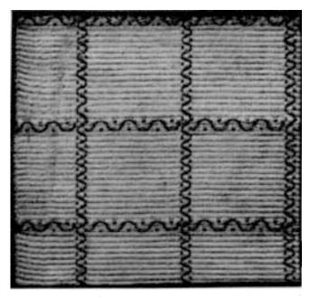
Pig. 602.—Piqué fabric figured both with extra coloured warp threads and picks of weft.
