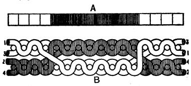
Fig. 649.—Sectional diagram showing construction of Kidderminster or Scotch carpet, Fig. 648...
