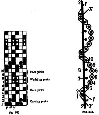
namely: two cutting picks, four face picks; two wadding picks and two face picks. (It should be observed at this stage, for the general guidance of students, that wadding picks should not be inserted until at least four face picks have followed the cutting picks of each rib. Otherwise, the wadding picks would prevent those face picks that follow them from approaching
