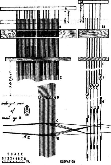
Fig. 553.—Compound presser harness, for damask weaving.
