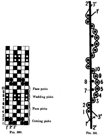
cuttings and "fine" cuttings respectively. If "coarse" cuttings are adopted, the furrows are relatively broad and shallow; whilst "fine" cuttings produce furrows of deeper and sharper delineation which, for reasons to be stated presently, imparts to the fabric a very superior effect.
