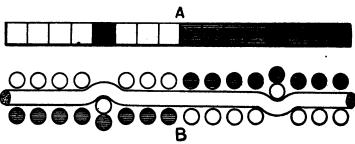
Fig. 646. —Transverse section of tapestry fabric containing two series of warp threads and one series of picks of weft,
