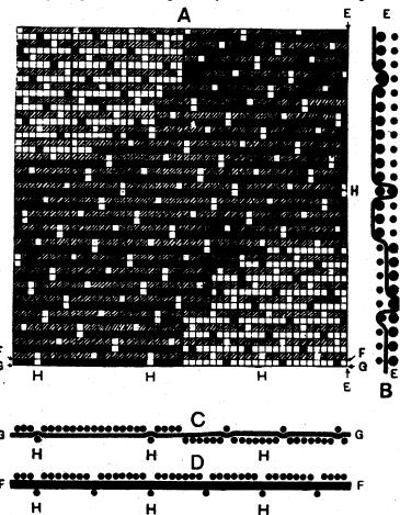
Fig. 569.—Showing actual structure of compound damask fabrics, Fig. 552. threads from the actual fabric, however, the binding warp threads reveal a more wavy appearance than that of the figuring threads, due to their greater rate of contraction during weaving.
