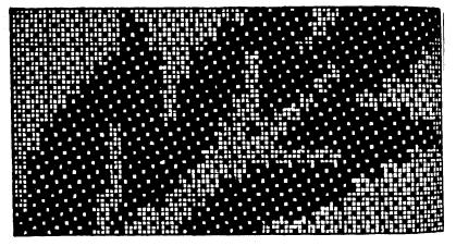
Fig. 565.—Showing structure of damask fabric with figuring as at A, Fig. 564.
