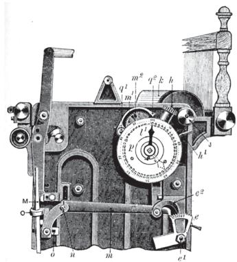
Fig. 50.—Automatic Measuring and Stop-motion.
