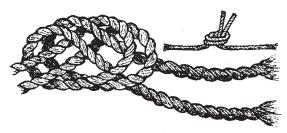
Fig. 33.—Winders' or Spoolers' Knot.
