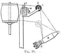
instead of both revolving together. Hence, the bobbins will revolve with a more or less eccentric and jerky movement, which causes a rattling noise, and also wears the bobbins on the inside, so that they eventually become too slack for the spindles of the ring-spinning frame, and have to be discarded.
