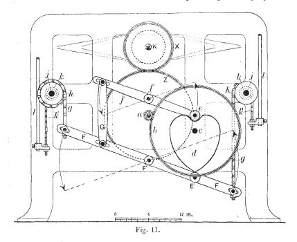
cams, their return upward movement is effected negatively by reason of the guide-rails descending by gravitation.
