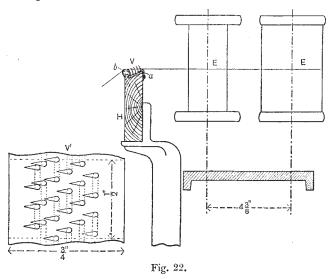
encounter any obstacles in the yarn, these latter are immediately caught by them and removed, or else their passage through the teeth is obstructed, and the defective threads break down.
