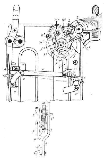
Fig. 51.—Automatic Measuring and Stop-motion.
