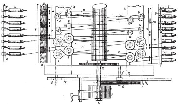
Fig. 5(b).—Cop or Bobbin Winding Machine (Part Plan).
