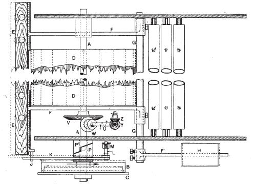
Fig. 44(b).—BEAM WARPING MACHINE (Part Plan).
