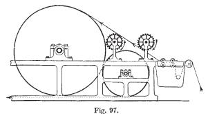
as the brushes, which are driven positively, revolve in the same direction as that in which the yarn travels, as indicated by arrows.
