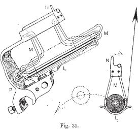
polished metal cradle or bedplate L, on which a ring spool simply rests by its own weight during winding. From the hollow crown of the bracket there are freely suspended two coppered tension or drag wires M, which hang one on each side of the spool, and against which they bear lightly.
