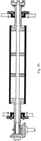
large notched discs. These are secured respectively to the sleeve bosses of the roller end-blocks, and also on one end of the roller shaft in one case; and on the inner end of the boss of the bevel wheel in the other case, so that when the respective clutches are in position the mortises and tenons of the complementary discs interlock quite freely.
