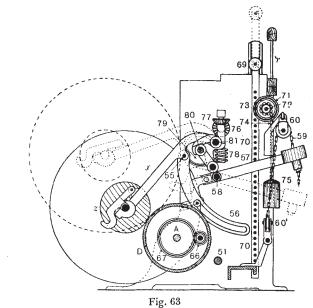
the footboard, the main driving belt passes from the loose pulley B, first on to the narrow-rimmed "slow-motion" pulley  $B^1$ , and thence on to the fast quick-driving pulley C, to put the machine into operation at full speed.
