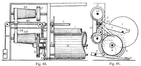
impart a differential velocity to the winding drum D. Motion is transmitted, through the medium of a belt 53, from the upper driving cone 52 to the lower driven cone  $52^1$ , and thence to the winding drum D by means of wheel gearing operating in conjunction with a frictional driving clutch B, C, mounted on the end of the drum shaft A.
