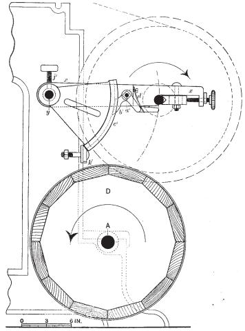
Fig. 58.—BEAM-RETAINING DEVICE.
