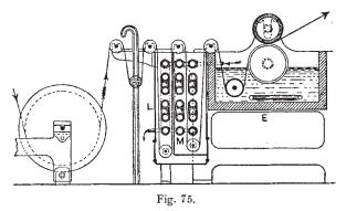
ments are furnished with several relays of steam-piping M, for the purpose of generating, within the chamber, hot and dry air, through which the sheet of yarn is conducted over guide rollers immediately before it enters the size-box E.
