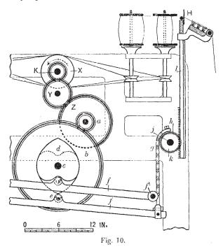
velocity of the latter being geared down in order to drive the spurwheel and the cams with a slow uniform velocity.
