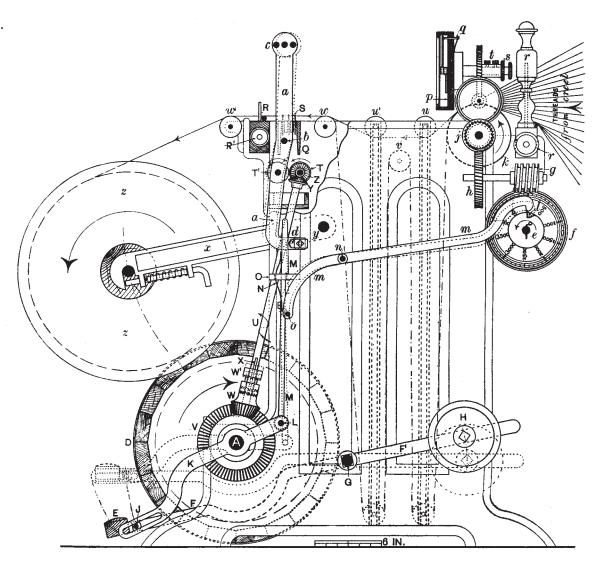
Fig. 44(a).—BEAM WARPING MACHINE (End Elevation).
