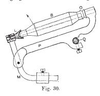
fixture P secured to a rod Q, on which it may be adjusted to any suitable inclination. In the upturned rear end of the bracket there is mounted a free spindle, which is furnished with a wharve O, and may be constructed with either a short or a long spindle shank on which a ring bobbin B is mounted with its lower end abutting against the spindle wharve. The bobbin is retained
