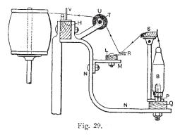
with which the threads are withdrawn as the warpers' bobbins gradually increase in girth.
