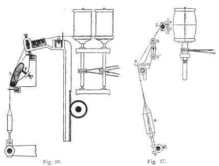
clearer-guide V on to the warpers' bobbin; or it may be passed immediately from the lower tension-bowl S<sup>1</sup> to the guide-rod, according to the degree of tensile strain it is desired to apply to the thread.
