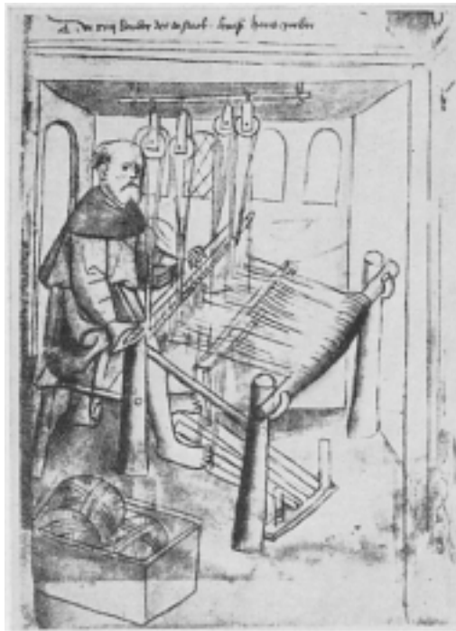
Old man at the loom. The shedding harness is suspended from the ceiling. The weaver works barefooted. Nuremberg painting, 1387.
