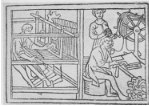
Treadle-loom with batten. From Rodericus Zamorensis, "Spiegel des menschlichen Lebens" (Mirror of Human Life). Augsburg 1477.
