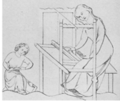
Fresco showing loom. Constance, early 14th century. The loom has the high frame form and is fitted with a batten. A child is spooling thread.
