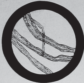
Jute (Fibres Magnified)
