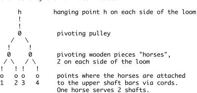
The hanging points should always be according to the ASCII sketch below. Connect each end of the horses with its own shaft. All cords must be equally long and hang straight down. Be careful to make it symmetrical, if the outer end of the horse is connected to shaft#4 on the left side, it must be so on the right side too. The inner end of the same horse is then connected to shaft#3. This part of the tie up may have to be redone for the next warp if the weaving is wide.
