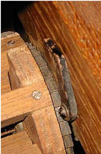
System of blocking of the front roller.
