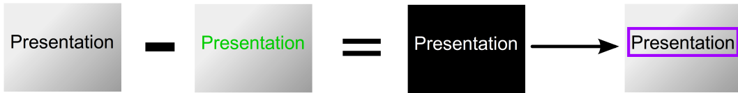
Figure 2.3: The bounding boxes of a particular word, sentence, or image can be found by making the color of the word unique and then taking the image difference. The differing pixels define the location of the word and a bounding box can be constructed from it.
