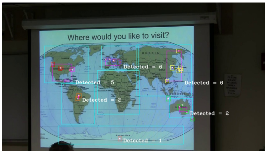
Figure 3.8: Output of our system tallying answers to geographical question. Our system makes it easy for a teacher to add regions (the light blue boxes) to a slide.
