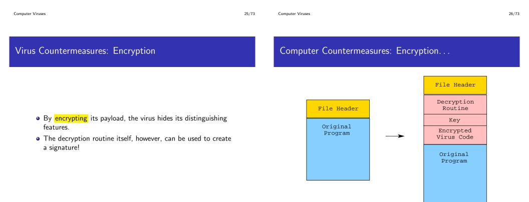
• Each variant is encrypted with a different key.
