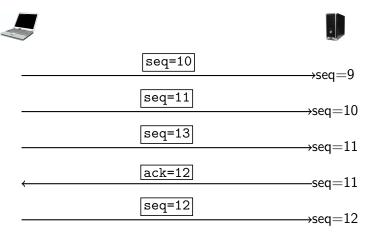
Receiver sends an acknowledgement package with the sequence number of the next payload byte it wants to receive.
