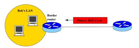
• Border router can block packets whose source address appears to be from inside the subnetwork, although they come from
