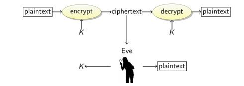
We have: the ciphertext of several messages that have been encrypted with the same key, *K*. We recover: the plaintexts, or *K*.
