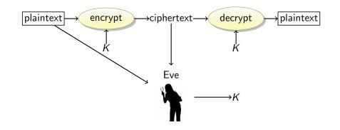
We have: the ciphertexts and corresponding plaintexts of several messages, all encrypted with the same key K. We recover: the key K.
