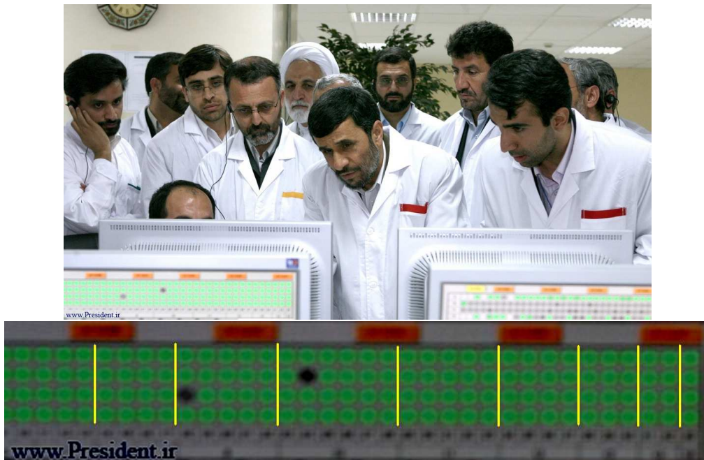
Figure 2: Iran's president revealed the cascade structure at Natanz: The dark lines at the bottom probably denote the division between stages; yellow lines have been added above them to make the division clearer. from right to left- 4, 8, 12, 16, 20, 24, 20, 16. (Photo: Office of the Presidency of the Islamic Republic of Iran)
