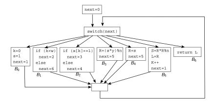
• Replacing 50% of the branches in three SPEC programs slows them down by a factor of 4 and increases their size by a factor of 2.
