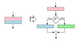
• Extend a loop condition *P* by conjoining it with an opaquely true predicate *P*<sup>T</sup>:
