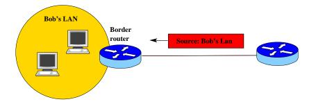
Border router can block packets whose source address appears to be from inside the subnetwork, although they come from outside the subnetwork.
