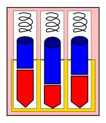
• In a locked lock, the driver pins are stuck between the sheer line, stopping the plug from rotating.
