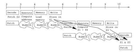
Some processors take care of data hazards themselves – the pipeline is stalled for a number of cycles until the hazard is resolved. This is like inserting one or more bubbles (NOPs) in the pipeline.
