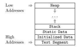
• The Text Segment holds the code (instructions) of the program. The Initialized Data segment holds strings, etc, that don't change. Static Data holds global variables. The Stack holds procedure activation records and the Heap dynamic data.
