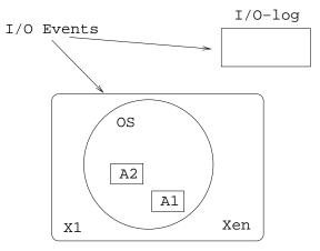
The OS (Linux) is running inside Xen, and two application processes A1 and A2 are running within the OS.
