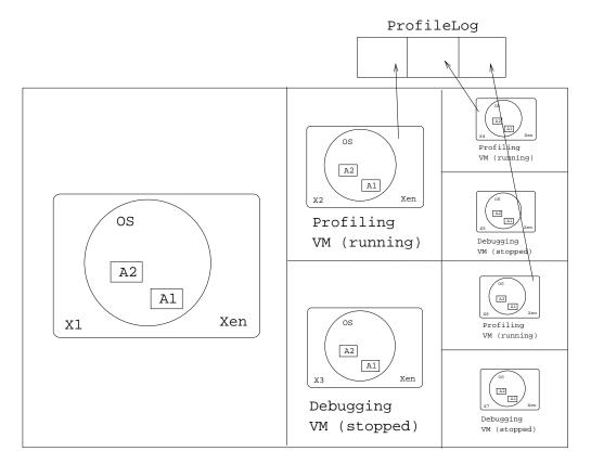
X4 and X6 are profiling VMs and run in the background, gathering performance data for some time period. If, for example, we create a new profiling VM every 10 seconds, X2 would collect from time 0 to 10, X4 from 10 to 20, and X6 from 30-40. At the end of their time period, they are killed off.
