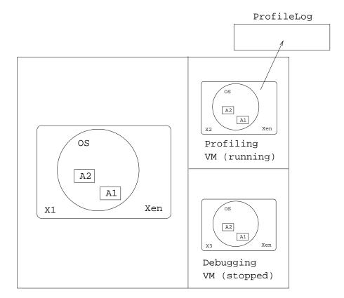
The idea is that X1 is the process with which the user interacts. It runs at near full speed, and collects very little data. What little information it collects it displays using simple counters and dials, to give the user a rough idea of what's going on.
