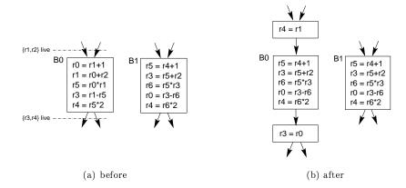
Fig. 2. Example of basic-block-level register renaming.
