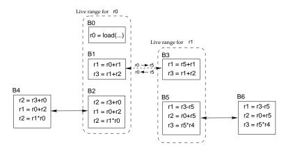
Fig. 3. Interference effects in live-range-level register renaming.
