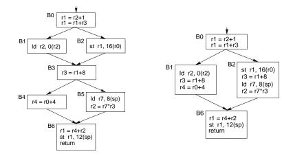
(b) Procedure obtained from the maximal (c) Procedure obtained after unmatching unprofitable instructions
