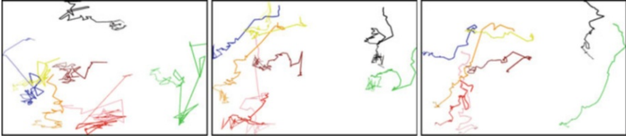
Fig. 10 Trajectories of randomly selected nodes with three different layout stability methods. ( Left ) independent layout with average distance traveled 21.41; ( Middle ) layout initialized with positions from the previous frame with average distance traveled 13.19; ( Right ) initialized positions and Procrustes transformation, with average distance traveled 8.43
