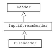
Since FileReader extends InputStreamReader, an instance of FileReader can also be assigned up to the Reader parameter in the BufferedReader constructor. Remember, assignment up the inheritance hierarchy is valid.
