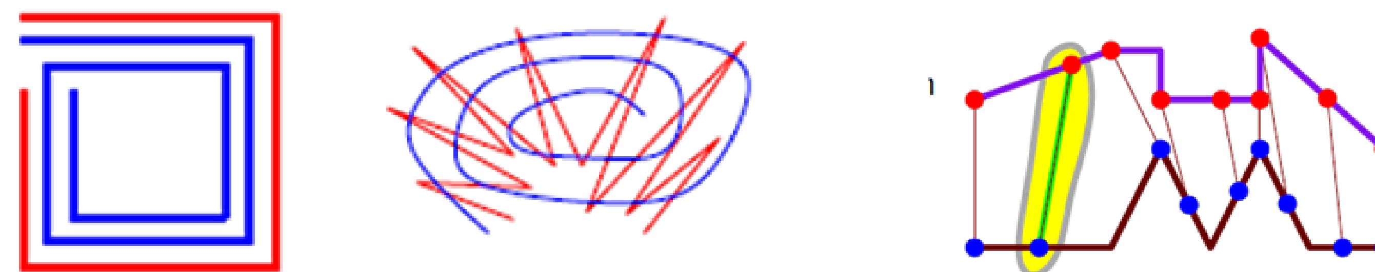
Two curves with small Hausdorff and large Fréchet distance. Fréchet distance minimizes leash length.
