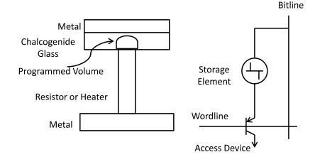
Figure 3.1: Structure of a PCM storage element.
