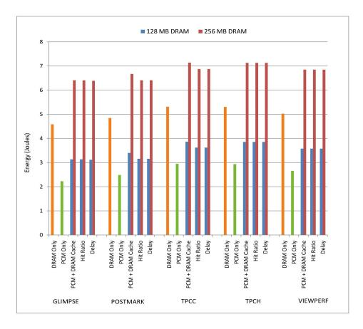
Figure 5.6: Memory energy characteristics of various benchmarks for different mechanisms when DRAM-cache size is increased from 128MB to 256MB
