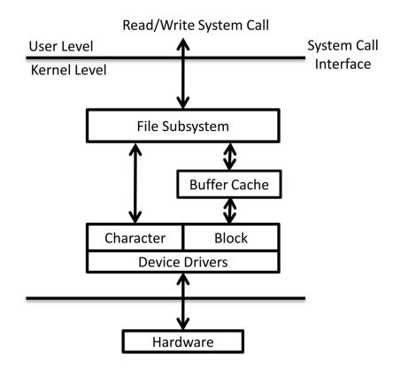
Figure 2.3: Position of the buffer cache during file-I/O handling
