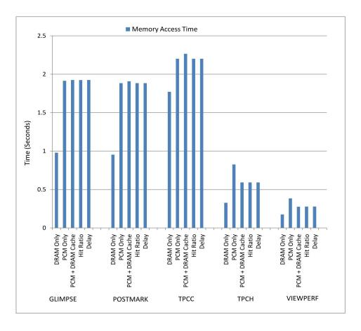
Figure 5.3: Memory access time of various benchmarks for different mechanisms.
