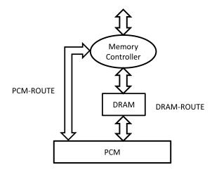
Figure 4.4: Buffer cache architecture for dynamic switching.
