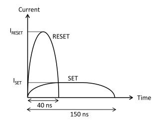
Figure 3.2: SET and RESET operations in PCM
