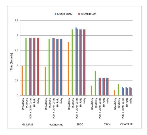
Figure 5.4: Memory access time of various benchmarks for different mechanisms when DRAM-cache size is increased from 128MB to 256MB
