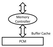
Figure 4.2: PCM as buffer cache
