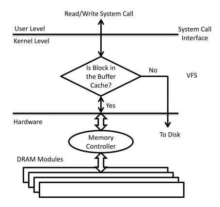
Figure 4.1: File-I/O system call handling
