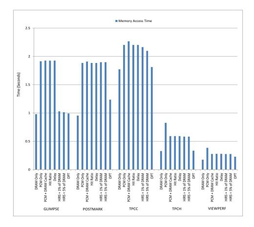
Figure 5.7: Memory access time of various benchmarks for different mechanisms with LIRS and OPT
