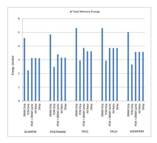
Figure 5.5: Memory energy requirements of various benchmarks for different mechanisms
