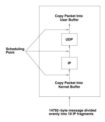
Figure 1: Structure of the UDP/IP Protocol Stack
