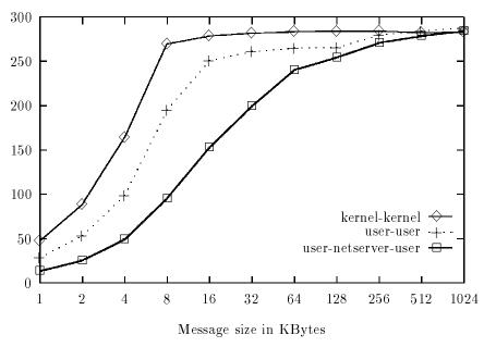
Figure 5: UDP/IP end-to-end throughput using cached, volatile fbufs
