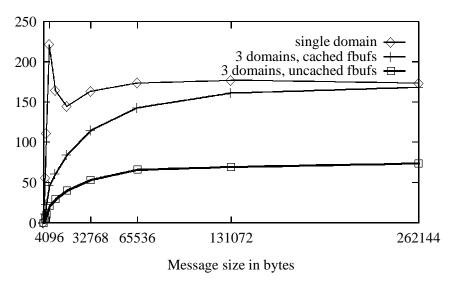
Figure 4: Throughput of a UDP/IP local loopback test
