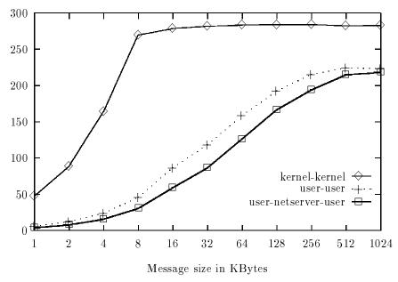
Figure 6: UDP/IP end-to-end throughput using uncached, non-volatile fbufs
