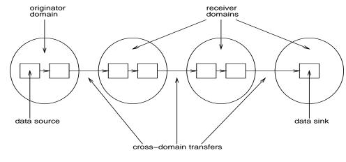
Figure 5.1: Layers Distributed over Multiple Protection Domains
