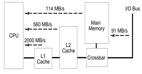
Figure 1.1: Block Diagram of a DEC 3000/600 AXP
