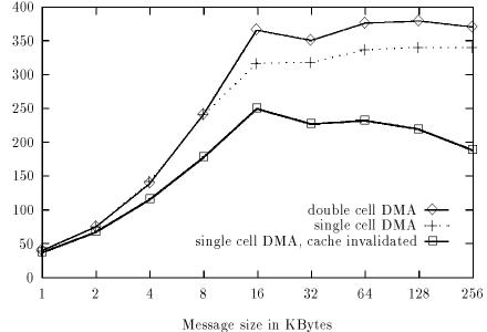
Figure 3.3: DEC 5000/200 UDP/IP/OSIRIS Receive Side Throughput
