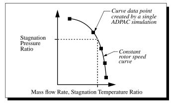
Figure 3: Single curve map for fan component
