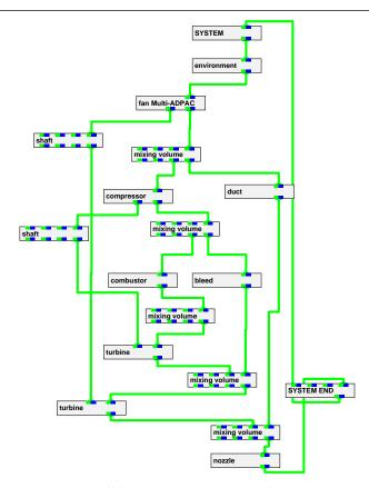
Figure 4: TESS engine model dataflow network
