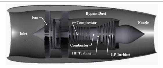
Figure 9: NASA's Energy Efficient Engine
