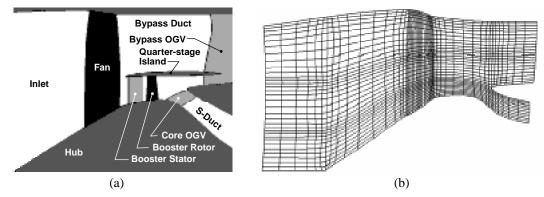
Figure 10: E<sup>3</sup> fan component (a) physical geometry; (b) computational grid
