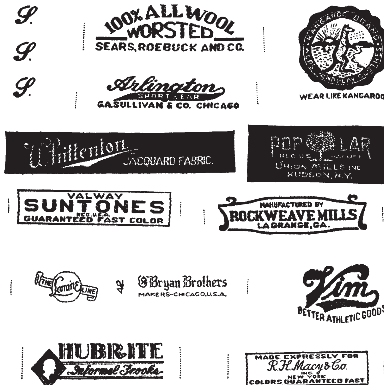
Figure 12 Labels Using one Extra Shuttle on Plain Weave Ground
