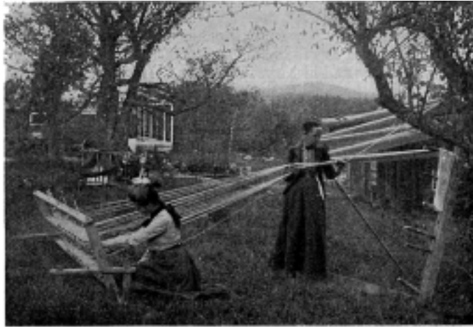
WARPIING THE WEB FOR A SABATOS RUG BEFORE HARNESSING IT TO THE LOOM.
