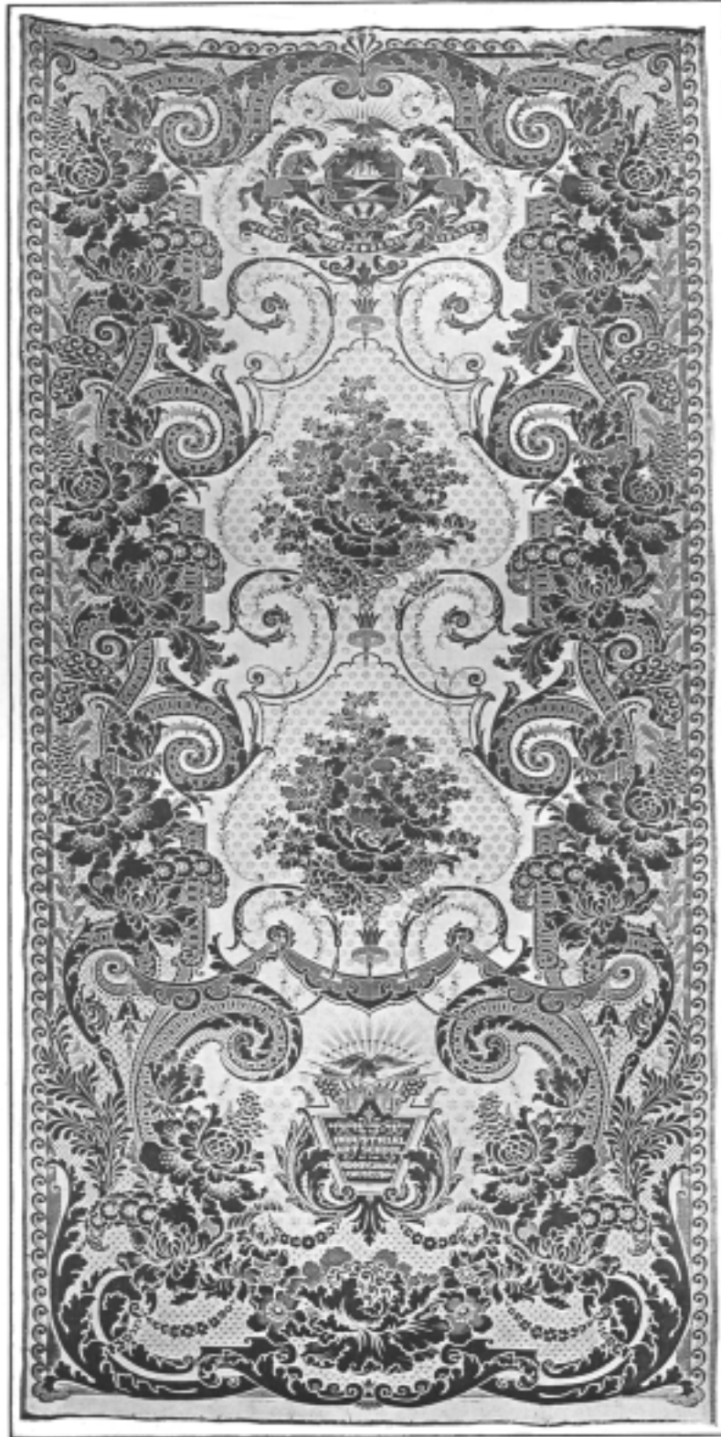
Silk Damask Curtain. Designed by William Laird Turner. Exhibited by the Philadelphia Textile School at the Chicago World's Fair. 210 ends per inch. 120 picks per inch. Pattern on design paper covered 174 square feet. 28,320 cards required to form the design on cloth, which placed end to end would extend a distance of 7\frac{3}{4} miles. The largest pattern designed in the United States, up to 1893.
