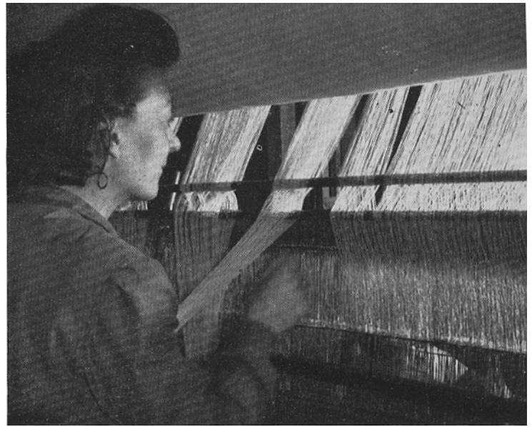
Drawing in. The operator pulls the warp ends through the healds and reed, so as to get the threads in the required order in the heald shafts.
