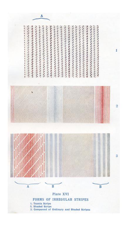
and the other of a light shade. Thus, a shaded stripe of blue may be produced in the Venetian twill by grouping blue and white threads together, according to the plan given below:—
