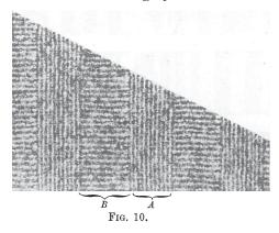
or covered by corresponding picks, it causes the same threads in A to float over the respective picks, producing this useful form of stripe, which is applicable to similar goods as those for which particulars are supplied in the preceding paragraph.
