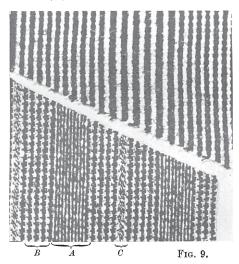
and-two and four-and-four stripings, grouped as sketched. Fig. 9 is a compound of hairline effect, one-and-one warping in the broken  $\frac{3}{1}$  twill, section A, and of two-and-two warping in the  $\frac{2}{2}$  twill, section B, with a fancy twist stripe, C, on the latter.
