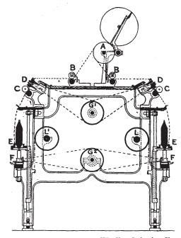
Fig.~89.~Sykes'~Continuous~Woollen~Spinning~Frame.  $G^1 = Cylinder~for~driving~the~Wharls.~G^2 = Cylinder~for~driving~the~Spindles.$
