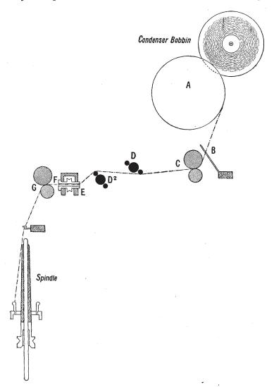
Fig. 90. Sectional Drawing showing the passage of the thread in the Continuous Woollen Frame (Sykes).
