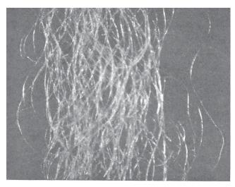
Fig. 91. Sliver from Condenser Bobbin.
