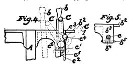
once springs in usual manner to the left into its dotted position shown in Fig. 4, and thereby permits the weight  $a^5$ , to turn the controlling member C into its extreme right-hand position and quickly apply the brake and stop the loom.
