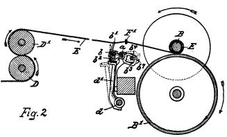
with is placed a rocking shaft d, rocking in suitable bearings in the frame of the machine. To this rocking shaft d, is secured at either side of the machine a vertically disposed rocking arm d', the two arms d'
