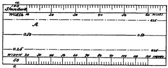
plate A and the length from the left end to the line on the a side of the plate marked "40." The piece cut to these dimensions is then weighed on grain-scales, and the number of grains the sample weighs—suppose it is twenty grains in this case—is divided into one hundred, the standard number, and the result, five, is the number of yards to the pound that the cloth weighs.
