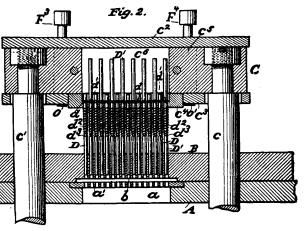
M, is provided with recesses, one of them,  $m^3$ , being of sufficient length to receive one group L, l, of the punches when the bar is in its normal position, and with recesses  $m^4$ , and  $m^5$ , separated by **2** partition m<sup>6</sup>, which is normally located between the
