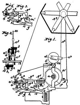
Fig. 1, in side elevation represents a sufficient portion of a spooling machine with the improvements added to enable its construction to be understood. Fig. 2, is a partial view of Fig. 1, looking from the left; and Fig. 3, is a detail with the snarling stop-lever shown omitted in the other figures.
