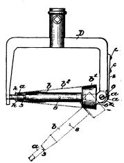
The sleeve b, is provided with an oil hole 8, for the introduction of oil between it and the dead spindle.
