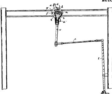
the box pattern-cylinder. Upright lever l, is actuated through connector c, from lever v, which is moved by cam m, integral with arms a, which are pulled up alternately as indicated by the punching of the Jacquard cards, by means of the cords d, which lead to lifter needles in the Jacquard.
