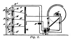
being then made between the strips K and I, by the thread-guide D, and the pivot H, together with the wires J and J', and the battery F. The threads B', after leaving the spools B, pass through the eyes D' and E, to the gatherer G, which holds the thread-guides D, in an uppermost position, so that the lower bent end of each thread-guide is a considerable distance away from the surface K' and the strip K, whereby the circuit remains open.
