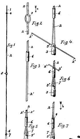
The heddle-wire 2 is made from a single piece or length of wire, which is bent upon itself at its middle portion intermediate its ends and then the bent or loop portion twisted to form an eye 4, through which the cord I, is passed to attach the heddle-wire thereto.
