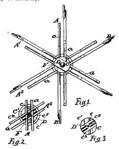
The manner of securing the skein-supports to the ends of the arms is as follows:—The skein-support B is of metal, and a ferrule is formed by striking half out of each side of the body of the support. The arm is
