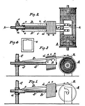
horizontal trunnions 0, are placed one on each side of the horizontal barrel of the socket J, to receive the rear ends of a double bar D, on the under side of which notches are made to fit on the trunnions 0. The front ends of the bar D, are secured by bolts to a frictionpad R, that rests on the surface of the yarn on the beam A. The object of the pad R is to make a friction on the yarm and to increase that friction and make
