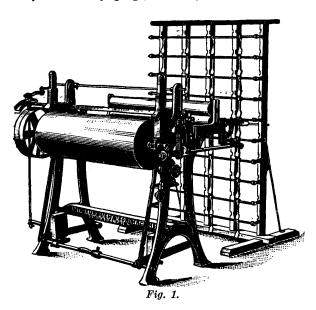
hook made of hardened and tempered steel, fastened to them by means of a small screw. These wire hooks are reversible, so that as the yarn cuts and wears them at one end, they can be turned and the other end used, or being merely fastened by a small screw, they can be easily and cheaply replaced with new ones. When an end breaks, the trap-guide falls and comes in contact with a constantly vibrating bar, and the machine is immediately stopped.
