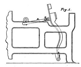
in each end to fit the crank-pin on the shaft and the wrist-pin on the lay, respectively, the pitmen being held to each pin by a **U**-shaped strap of leather or metal straddling the end of the pitman and fastened by a transverse bolt. The constant and severe shock produced by the successive thrust and pull tends to split the ends of the pitmen, necessitating frequent repairs. The new pitman aims to overcome this difficulty and expense.
