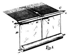
Of the accompanying illustrations, Fig. 1 is a perspective view of a cloth-roll on a loom, showing the protection-rail and the cutter/carried on the edges of the cloth. Fig. 2 is a perspective view of the cutter removed.
