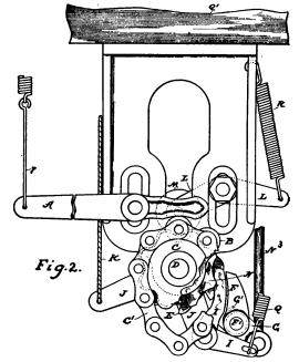
to be raised in the working of the Jacquard mechanism, and thereby the bent lever J is moved so as to draw the pawl-lifter I out of the way and permit pawl F to engage with a tooth of rachet E.
