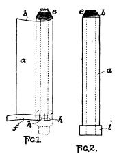
connecting the end of the strip which forms the peripheral flange or base. Fig. 2 is a side view of a finished bobbin.
