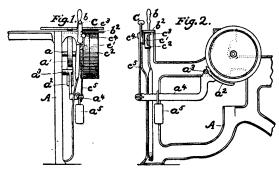
the brake when the shipper is moved to stop the loom and capable of automatically releasing the brake when the shipper is restored to running position, and, further, having an independent movement to release the brake while the loom is stopped.
