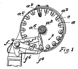
a series of radial guides which receive the slotted heads of the carriers. They also shaped the heads of the carriers so as to present two secant surfaces, which surfaces, when the carriers meet and are being pushed together, act one on the other to prevent any rotation of the carriers.
