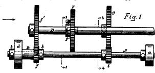
spinning machines or machinery generally in which it is desirable that a shaft shall move faster at one time than at another, or faster at one part of each revolution than at another part of the same revolution.
