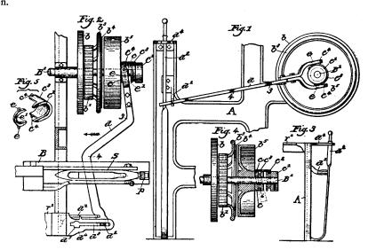
own resiliency tending to normally remain in its outermost positions, Figs. 2, and 3, the said shipper working in the usual slot  $d^3$  in the catch-plate  $d^4$ , the latter being provided with a holding-notch  $d^5$ . (See Fig. 2.)
