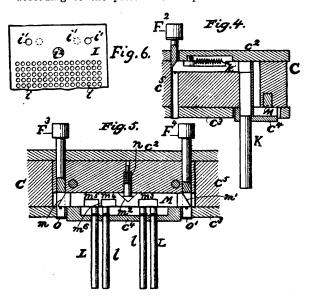
in operative adjustment by the depression of the proper keys F, F', and the head C, with the punches locked, is then depressed, forcing the punches through the card as it rests upon the perforated plate a'. As soon as the head C, is returned to the upper limit
