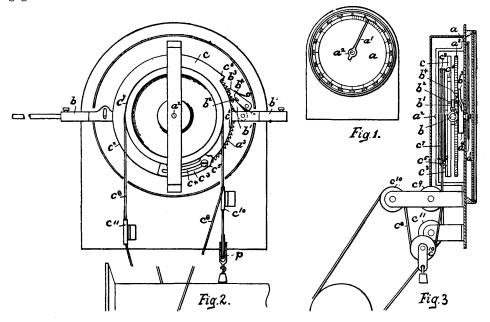
The trip-wheel is made to revolve continuously at a speed corresponding to the speed of the fabric through the loom, while the vibrating-lever b is connected so as to vibrate each time the shuttle of the loom is operated. The depressed portion of the trip-wheel corresponds in length to a certain length of cloth, so that the number of vibrations which the shuttle makes in this space will represent the number of picks or threads which are woven into a certain length of the fabric.
