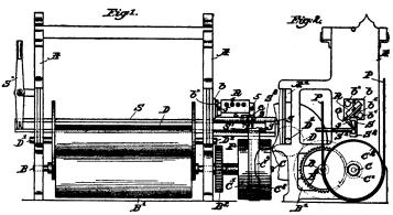
series of openings therein, beneath each of which is located a disk, each disk provided with the digits and zero in well-known manner, the complete rotation of one dial turning the next succeeding one through one step.
