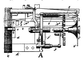
is an enlarged sectional view of the temple-head, showing the manner of attaching the filling-cutter. Fig. D is a transverse section thereof on the line x-x,
