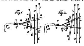
cords are applied in the harness-mechanism for raising or lowering the frame I, and as this movement takes place, the frame H and the vertical bars 10 of the distenders G, swing upon the pivots 12, so as to allow the parts easily to assume the proper positions as the
