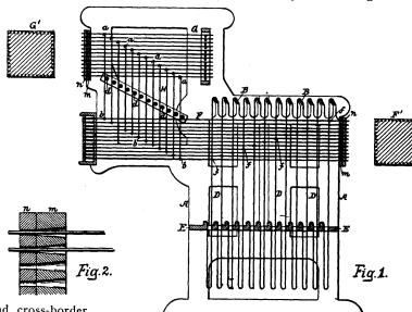
respectively at the right and left-hand sides, or rather at the front and rear of the machine. The two sets of needles are connected for joint operation by means of levers H, which consist of wires having hooked upper ends engaging with eyes a, upon the needles G, the lower ends of the wires engaging with eyes b, upon the needles F, said levers having their fulcrums upon transverse rods d, suitably mounted upon the fixed frame of the machine.
