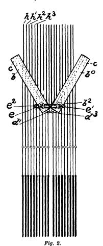
In the grooves a', and b', is arranged the comberboard proper, consisting of a series of two or more sections d, d',  $d^s$ , and  $d^s$ , connected together by threads
