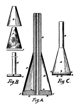
and base of the bobbin, renders said bobbin preferable to one made entirely of sheet-metal by reason of its less weight and cost, and by preventing injury to the yarn, which is likely to result from contact with said sheet-metal surface, the latter being liable to oxidize in the damp atmosphere of a mill, or by reason of the wetting of the bobbin in some of the various processes of manufacture in which it is to be used. (R. Blackburn, Nottingham, England.)
