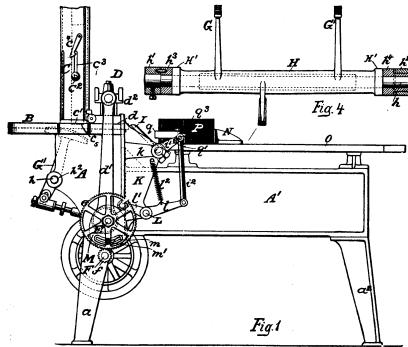
rock the shaft i, and hence the rest I, at the proper moment during the rotation of the wheel The vibrating lever pivoted at L, is operated in a direction to return the rest I, by means of a spring  $l^2$ , connected at one end with the arm l, and at its opposite end with
