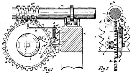
its return movement. This is an important feature of the new mechanism, i. e., that the striking mechanism can be operated having the reel-supporting shaft rotating in either direction, since in older mechanisms where the reel-supporting shaft is arranged to rotate only in one direction, frequent breakage is caused by reversing the rotation of said reel-supporting shaft. (B. Eastwood, Paterson, N. J.)
