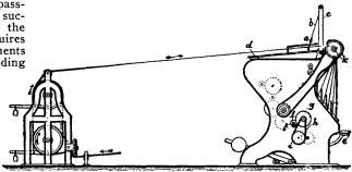
g, which rests on the shaft between the nut on the end of the shaft and the pinion f, so that when the stop-link is removed, the pinion f, can be drawn outward, and the pinion disconnected from the gear l, thereby disconnecting the spindle-driving mechanism from the cop-building mechanism and permitting:
