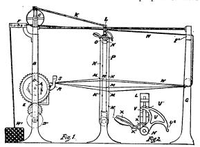
ing the warp-threads and thus by the use of this machine retain the major portion of the size deposited on the warp-threads, thereby preserving the strength and weaving qualities of the warp.
