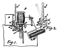
above the top of the spool to form a handle  $d^a$ . Normally the handle  $d^a$ , occupies a substantially vertical position, as shown in full lines, Fig. 2, the pin or stud d' then resting against the shoulder 2 of the lifter-bar  $a^a$ , the shoulder being concaved as shown in Fig. 2, to form a species of lock, the roll  $a^a$ , being at
