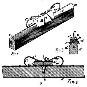
is placed such an improved thread-guide. Fig. 2 is a longitudinal sectional view of a portion of the bar and of the thread-guide; Fig. 3 is a transverse sec-
