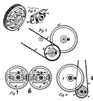
the others being omitted in order to avoid confusion. Fig. 3, is a transverse section on the line 3-3, Fig. 1, but showing only the second pair of gears. Fig. 4, is a
