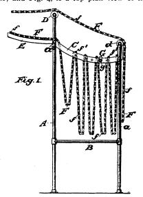
The support comprises four standards, those at the rear being denoted, respectively, by A, A', and those at the front being denoted by a, a', the standards being
