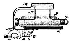
check the movement of the bobbin, and should the bobbin escape over the corners it will rest upon the wings, and under the action of the guards will be pushed back again into the cavity. In this way the wings prevent the escape of the bobbin from the pan. (Draper Co.)
