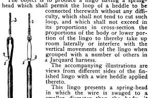
This lingo presents a spring-head in which the wire is swaged to a smaller diameter than the body, it having a flattened tongue I, an oppos-ing flattened back portion 2, and a neck portion of circular cross-section extending throughout the bend of the neck. The neck portion is wholly free from any projection or edge such as would tend to cut the loop of a heddle. At 3, is shown part of a heddle which is connected with the lingo. (Crompton and Knowles Loom
