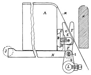
a spring (not shown). N is a board which extends the width of the breast-beam and is held in place by a pair of brackets which are not shown in the illustration. (Crompton and Knowles Loom Works.)
