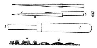
Fig. 113.—Knife for cutting the cords:—the broken ends b, b, should be joined. Fig. 114.—Representation of the cords.
