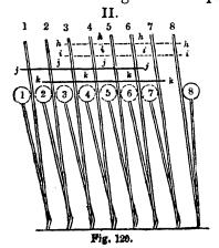
left of their respective warp-threads. The pusher-bar j, moves one side-step to the right; the guide-bar does the same; all the other bars remain unmoved. Fig. 121 shows the position of the parts after the third movement. The warp-threads are once more vertical, and one-half of the bobbin-carriages are placed upon the front bolt, and one-half upon the back bolt; the front and back pushers stand in pairs over each other.
