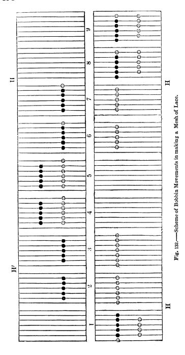
odd carriage in No.1  $\phi$  has advanced one step to the right, and become one of the front line; one of the back line  $\phi$  has advanced one step to the left, and has become the odd carriage; and one of the front ones  $\phi$  has gone over to the back line on the right. The bobbins and carriages throughout the whole width of the machine have thus crossed each other's course, and completed the mesh of net.
