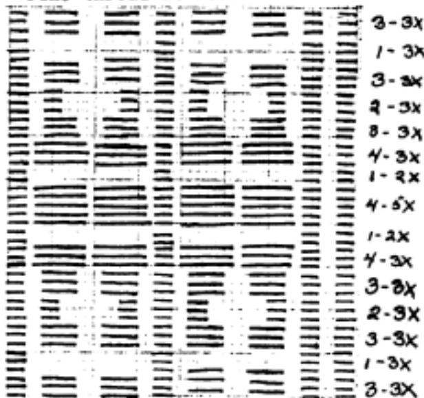
Drawing showing woven effect of draft No. I. The threads on stick No.1 of this draft pick up 15, and so this skip is a very long one, so it is best to set this in fine thread at about 30 to the inch.
