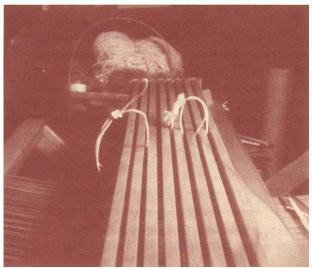
Cord loops for lifting harnesses by hand.
