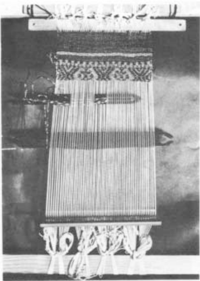
Figure No. 3—Photograph of simple heddle loom ready for weaving.
