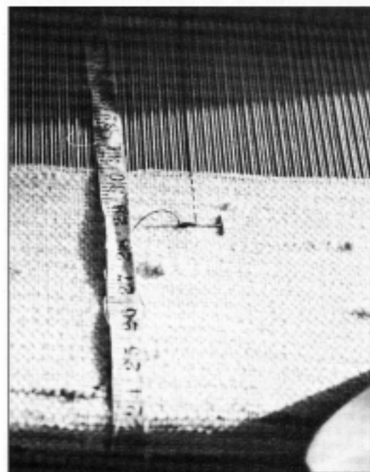
Method 1: Working the slit with two shuttles.
