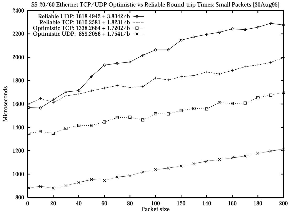
Figure 4.10: Ping-Pong Tests of Low-level Interfaces: Small Packets
