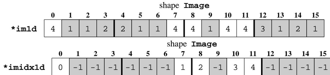
Figure 3.13: Elevation and Index Data in One Dimension
