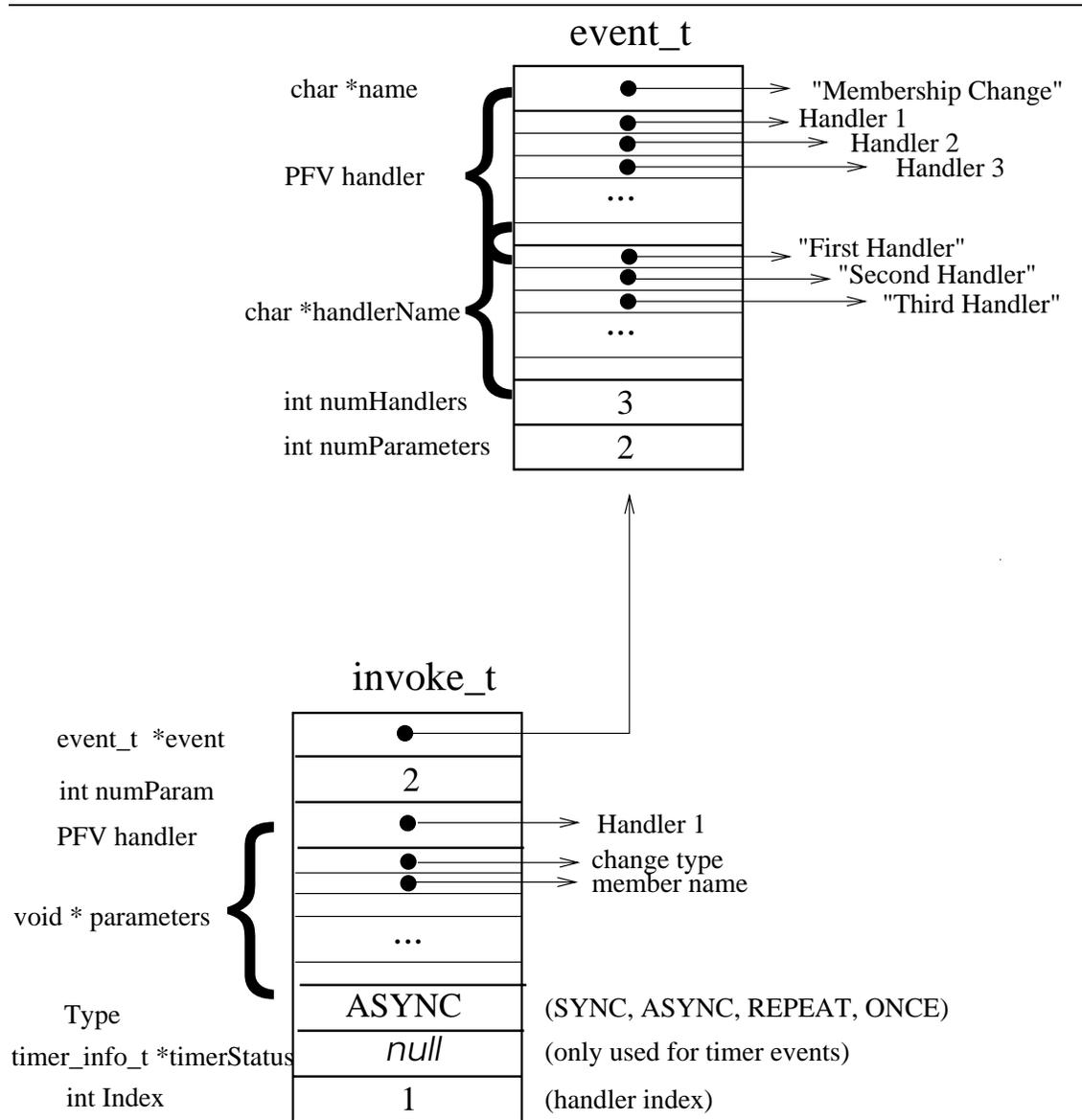
Figure 4.2: Event invocation structure with event description structure.
