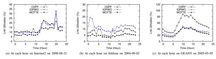
Fig. 5. Maximal Link Utilization of MCFTE and IGP Weight Optimization
