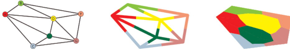
Fig. 1. Given a drawing of a planar graph(a), we apportion the edges to the endpoints by cutting each edge in half (b), and then apportion the faces to form polygons (c).
